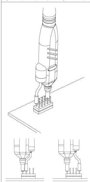
Using two square-in pin adapters for ground and signal, the probe can be connected directly to a pin strip.
