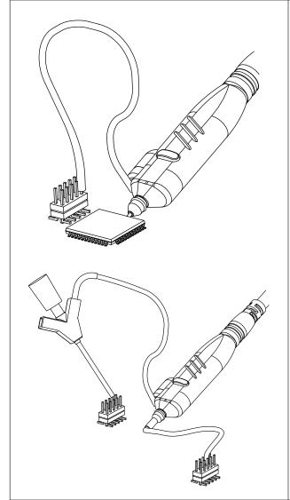
The lead provides a flexible connection to the DUT. It is plugged onto a pin on the DUT and can be used to connect either the signal socket or the ground socket. In addition, it allows micro and mini clips to be connected to the probe.
