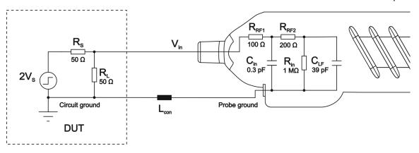
Figure 4-2: Equivalent circuit model of the R&S RT-ZS60 probe
