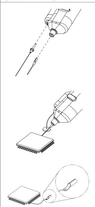
Using two solder-in pins for ground and signal, the R&S RT-ZS60 is soldered directly into the circuit.
