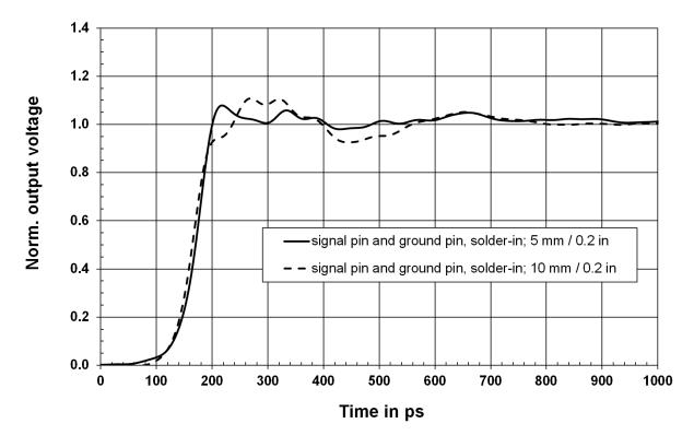
Figure 4-7: Step response of the R&S RT-ZS60 with a type 2 connection
