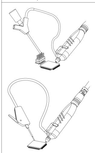
The mini clip is designed for probing large IC pins, wires and through-hole components.
