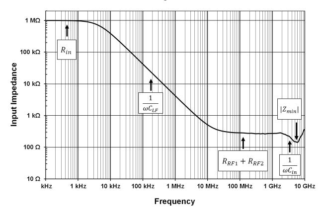
Figure 4-9: Magnitude of the input impedance of the R&S RT-ZS60 probe as a function of frequency
