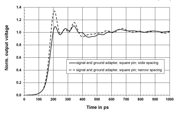
Figure 4-8: Step response of the R&S RT-ZS60 with a type 3 connection
