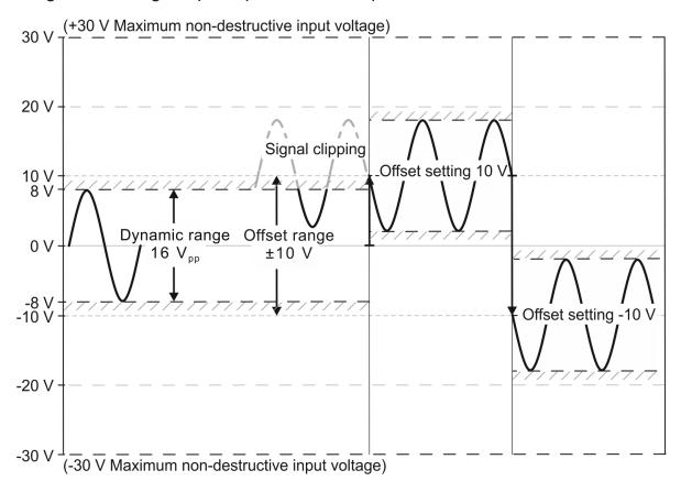
Figure 4-1: Offset compensation voltage and dynamic range
