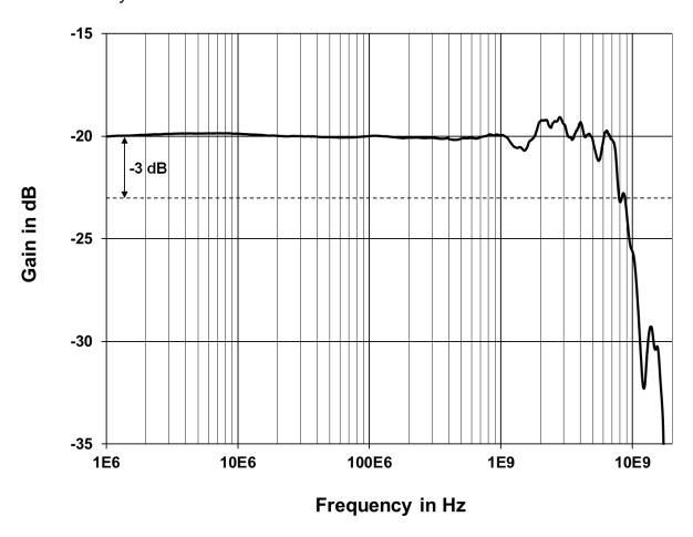
Figure 4-3: Amplitude/frequency response of the R&S RT-ZS60
