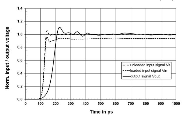
Figure 4-11: Unloaded and loaded input signal and step response using the example of R&S RT-ZS60
