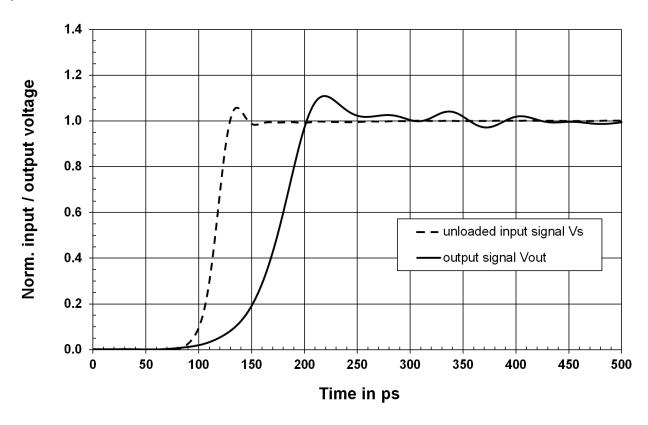
Figure 4-4: Step response of the R&S RT-ZS60
