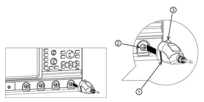
Figure 3-1: Connecting the probe to the Rohde & Schwarz oscilloscope
