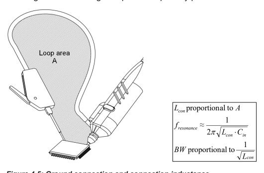
Figure 4-5: Ground connection and connection inductance
