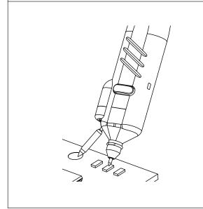
Using the signal pin and ground pin, manual measurements can be performed without or with only minor limitation of the measurement bandwith. Best results are achieved if the distance between signal and ground is small.
