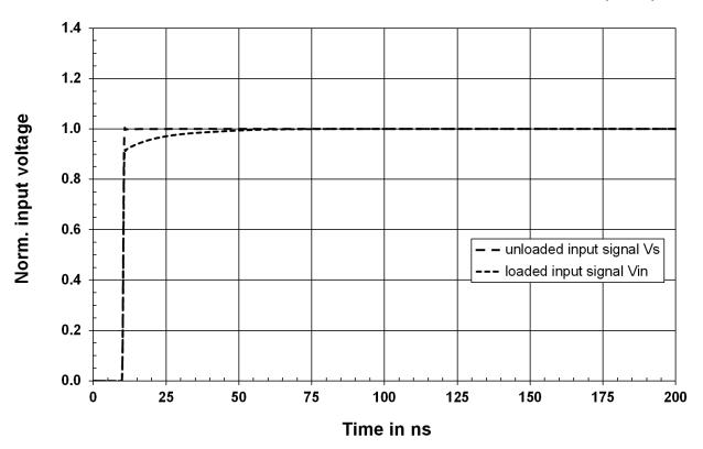
Figure 4-10: Signal loading caused by the R&S RT-ZS60 probe at an effective source impedance of 25  $\Omega$
