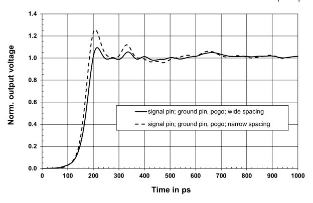
Figure 4-6: Step response of the R&S RT-ZS60 with a type 1 connection
