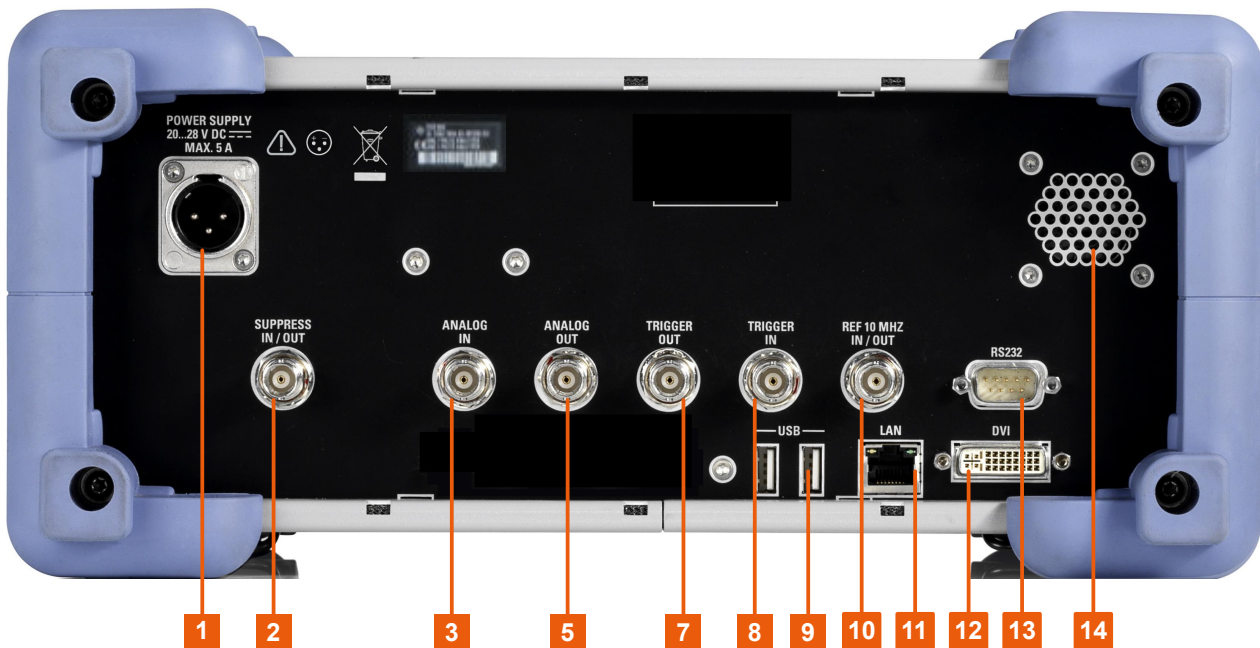
Figure 4-2: Rear panel view of the R&S EDS300
