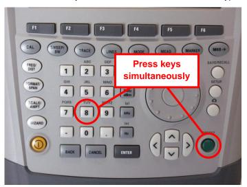
2. Switch the instrument on and keep PRESET and 8 pressed for at least 5 seconds after the startup screen has appeared on the screen.
