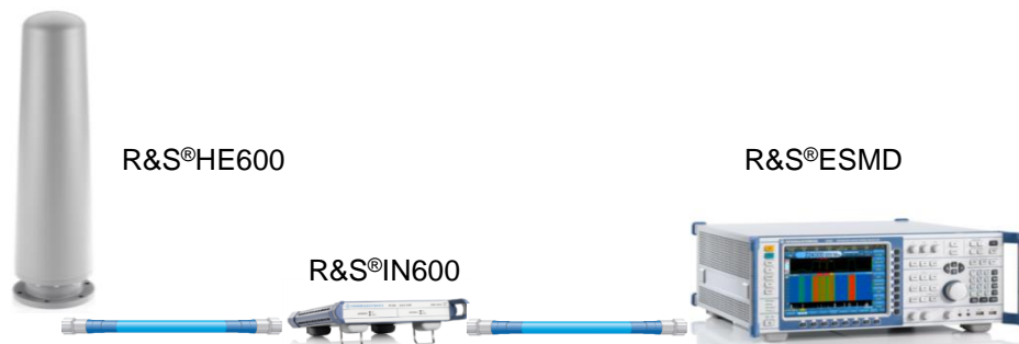
Figure 14: Monitoring system setup with an active antenna and bias unit
